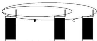
Let us consider that A and B both sending with the same transmission power. When the signal strength decreases proportionally to the square of the distance B's signal drowns out A's signal .As a result 'C' cannot receive 'A's transmission.
