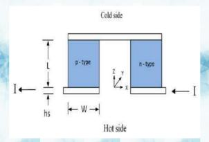
The dimensions of the semiconductor elements are as follows length and width are one millimetre and the cross sectional area is one square millimetre. The cold end
